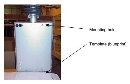
3. Install the Night Scan Chief base unit by using four (4) 5/16-inch 303 stainless steel bolts, washers and nuts (not supplied). The length of the 5/16-inch bolts will be determined by the thickness of the roof plus one inch for the material thickness of the Night Scan Chief unit. Apply a quality silicon sealant around the bolts during installation.
