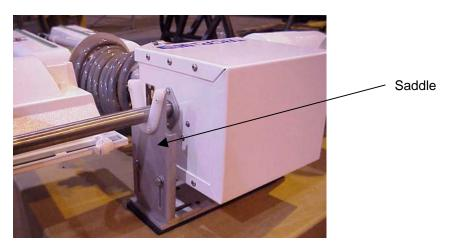
2. Rest the RCP shafts into the top of the saddles, placing each saddle between the RCP head and the light fixtures.
