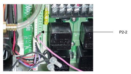
3. Route other end of wire to power common pin (P2-6) on the control board.
