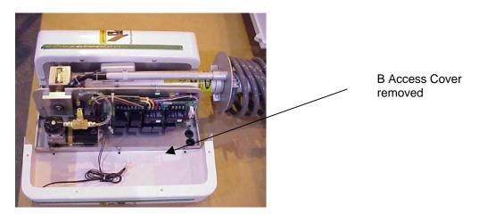
2. Feed two (2) 12/24V DC wires through one of the grommet holes in the bottom of the base unit
