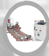
Self-developed winch load testing machine with the max capacity of 20000lbs.
